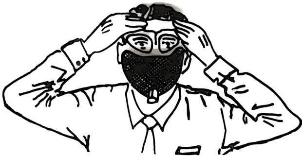
STEP 3 SMOOTH OUT EDGES OF MASK TO PROPER FIT ON FACE. ADJUST HEAD HARNES STRAPS IF NECESSARY
